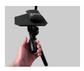
When engaging your target, we recommend tightening the fluid head when you are just below your target. You will then lightly push down on the handle and push forward with your gun to make minor aiming adjustments. See YouTube videos for more suggestions
